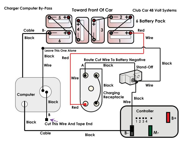
On the back of the charging receptacle locate the long black 12 gauge wire (A) that routes to the computer. Cut this wire as close to the computer as possible and tape up bare end (B) going into computer. Install a 5/16" ring terminal on the long 12 gauge receptacle wire and route to either B- on battery pack main negative terminal. Or route the wire to B- on controller or negative Stand-Off terminal (if used).
